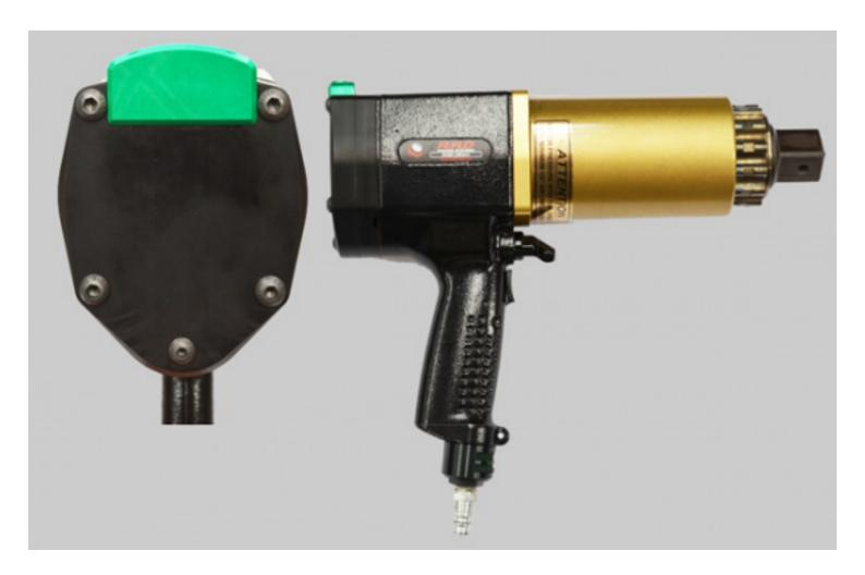
The Operator Safety Valve "OSV" is a retro fit accessory that can be fitted to any pneumatic RAD tool and is guaranteed to keep the operators hands away from the reaction arm which equates for 99% of pinch point injuries. once the "OSV" is fitted to the tool the operator can only operate the unit using both hands, one on the conventional trigger and the other on the OSV secondary trigger, located at the back of the tool ensuring both hands are away from the reaction arm.
